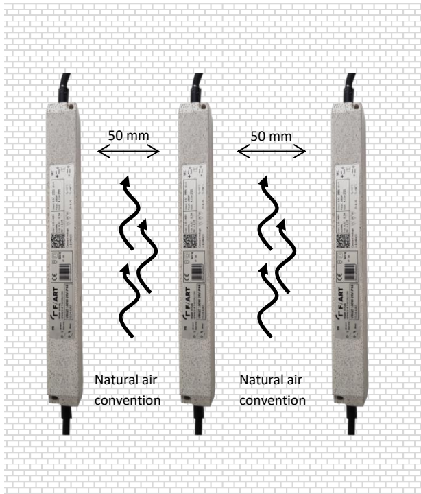
Figure 1 recommended VERTICAL installation diagram for a proper heating dissipation
